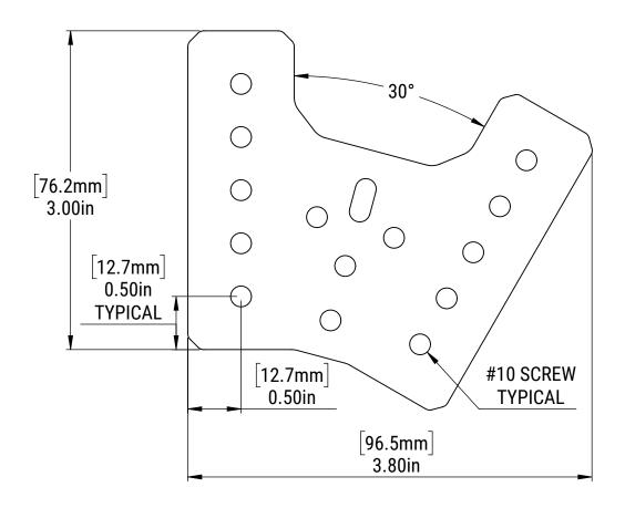
MM SHEET TOLERANCES:  $X \pm 0.50$  MM  $X.X \pm 0.10$  MM  $X.XX \pm 0.05$  MM ANGLES  $\pm 2^{\circ}$
