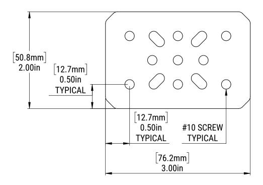
MM SHEET TOLERANCES:  $X \pm 0.50$  MM  $X.X \pm 0.10$  MM  $X.XX \pm 0.05$  MM ANGLES  $\pm 2^{\circ}$
