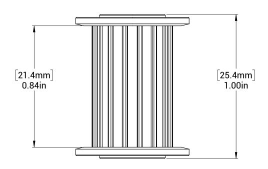
MM SHEET TOLERANCES:  $X \pm 0.50$  MM  $X.X \pm 0.10$  MM  $X.XX \pm 0.05$  MM ANGLES  $\pm 2^{\circ}$
