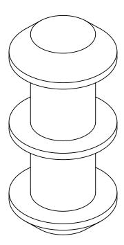
MM SHEET TOLERANCES: X ± 0.50 MM X.X ± 0.10 MM X.XX ± 0.05 MM ANGLES ± 2° INCH SHEET TOLERANCES: X ± 0.1 IN X.X ± 0.02 IN X.XX ± 0.004 IN X.XXX ± 0.002 IN ANGLES ± 2° MATERIAL: **BRASS**
